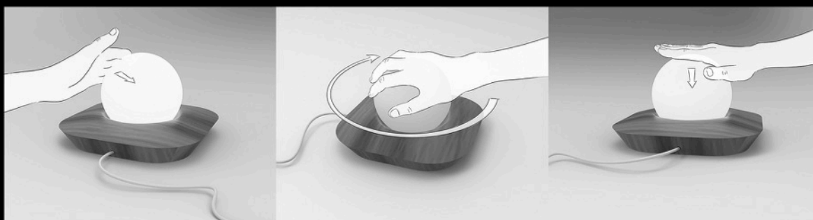
f) tangible interaction design: slapping the bowl skips a task, grinding the bowl in a circular motion deletes a task, and pressing the bowl for several seconds declares a task finished.
